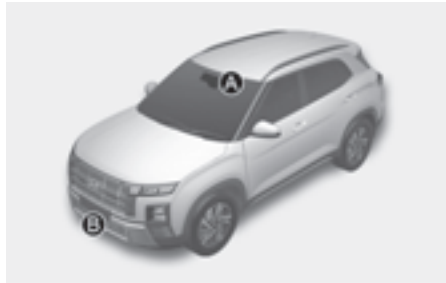
[A] Front view camera [B] Front radar
